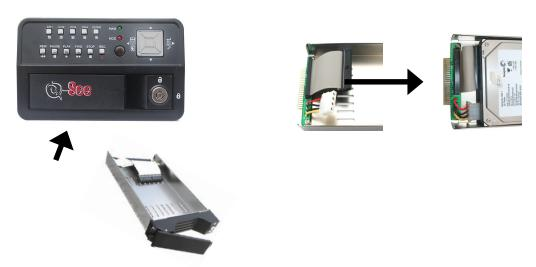
**CAUTION:** The wedge at the end of the cartridge handle must be fully inserted into the compartment; otherwise the cartridge will not be able to insert into the DVR firmly, it could also cause damage by scraping the body of the DVR.
